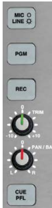
Fig 2-3: Mic/Line Channel Strip.
