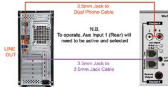
Fig 2-10: Connection Diagram For Channel 9 For PC VOIP Application.
