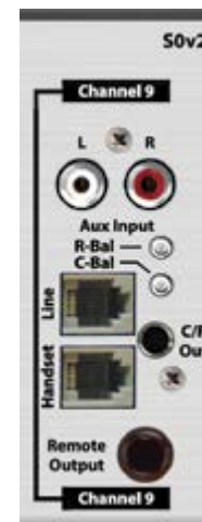
Fig 2-8: Channel 9 Rear Panel Connectors.
