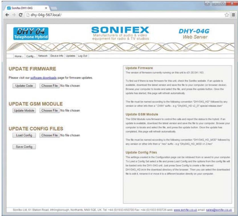
Figure 6-9: Updates Page – to update the system firmware and load/save configuration files
