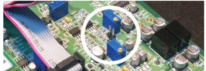
Figure 2-2: Internal Position of Jumper J1
