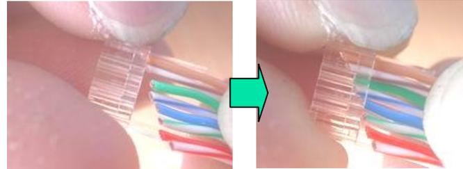
6. Cut the Balance Wires
