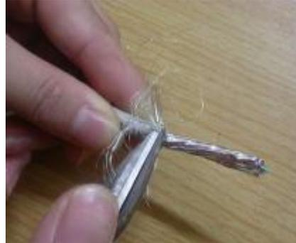
3. Cut foil for 4 Pair Wires
