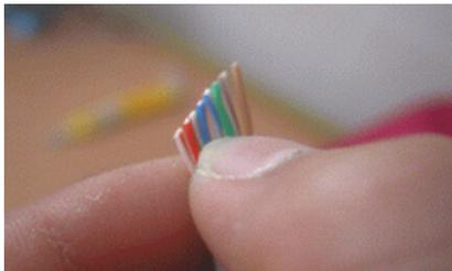
Remark: Cut the wires with a scissors in a oblique angle. It will be easier to insert the wires into loading bar.
