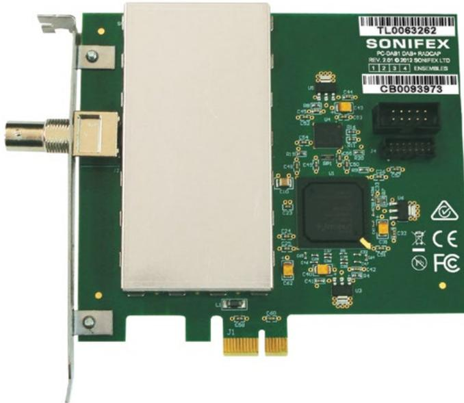
The PCI DAB+/DAB radio capture card receives and decodes the entire contents of up to four DAB+/DAB ensembles, rendering each audio service as a virtual Windows audio capture device for use with multi-channel recording or monitoring software.
