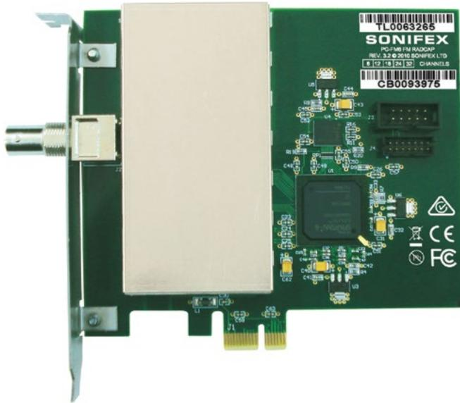
The FM Radcap PCIe is a radio capture card designed for simultaneous recording of multiple radio stations. The frequency of each station is set in software and its audio appears as a standard Windows audio input device. RDS decoding is also supported.
