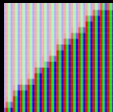
Non pixel mapped video can deliver soft edges
