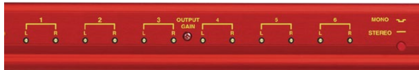
Fig 5-5: RB-DA6RG Front Panel Output Gain Controls and Stereo/Mono Switch
