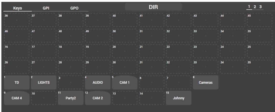
Figure 8 - Keys display for MP-16 with two Expansion Panels paired
