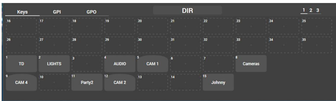
Figure 7 - Keys display for MP-16 with one Expansion Panel paired
