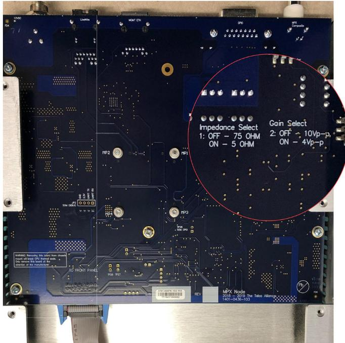
The Impedance / Gain switches are located under the chassis, and are more challenging to adjust. Magnification is recommended.
