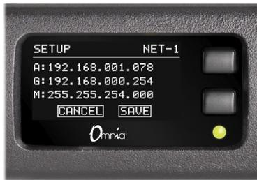
5. Use the upper front panel button to change values, and the lower button to advance to the next field. To save changes, advance to the SAVE field and press the upper button.
