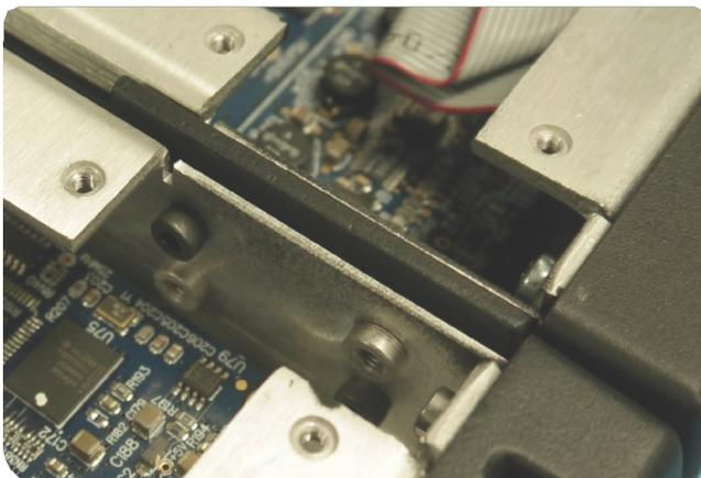
Replace the lids on the Nodes. Secure the short rack ears to either side of the two units.
