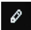
Pages 4 displays this “Pencil” icon, indicating you can edit the NET1 IP address settings from the front panel. For access, press and hold the bottom button for 10 seconds until the IP Setup screen appears.
