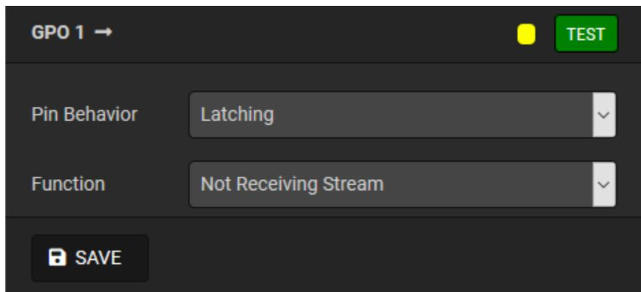
1. A drop-down menu for Pin Behavior selects between Latching and Pulse. For GPO's, pulse duration can be set to 250ms, 500ms, and 1 second, providing maximum flexibility in triggering other equipment.
