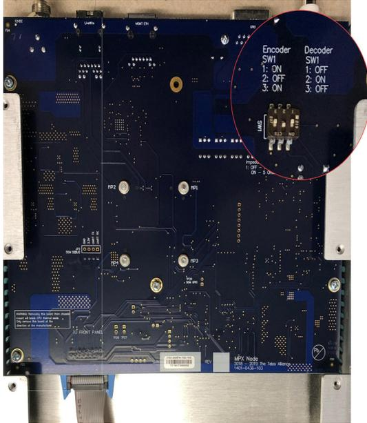
When adjusting, we recommend using a magnifying glass and a small flat screwdriver to move switches. This photo depicts an MPX Node set as a Decoder, with switches set 1:Off, 2:On, 3:Off
