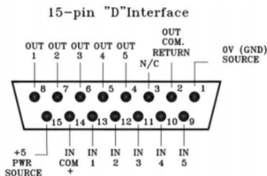
There are two options for wiring up the GPIO connector.
