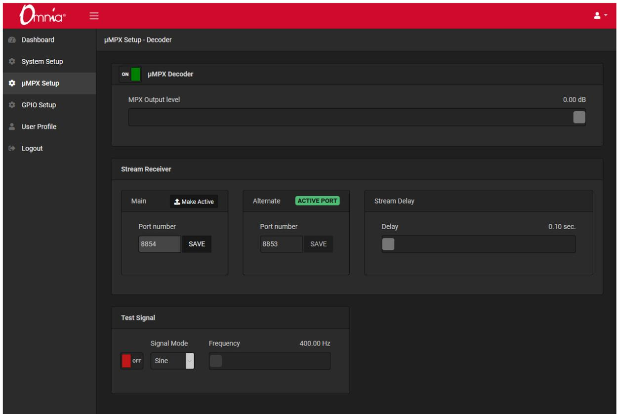
To configure decoding, go to the μMPX Setup page:
