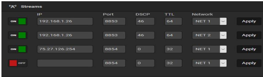
If you want to send more streams from your Encoder, you will need an extended license. Encoders can push up to 16 Unicast streams. Please note that the more Unicast streams you send, the more network uplink bandwidth is required, so be certain to factor in any bandwidth constraints
