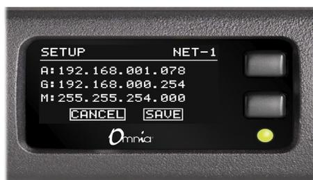
Use the top button to change values, and the bottom button to advance to the next field. To save changes, advance to the SAVE field and press the top button.
