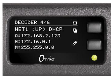
4. If you don't have a DHCP server on your network, you can enter a static IP address from the front panel. Press and hold the bottom front panel button for 10 seconds until you see the Setup page.
