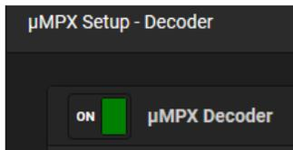
The μMPX bitrate is set by the Encoder, and there are no controls or displays on the Decoder to register rates.
