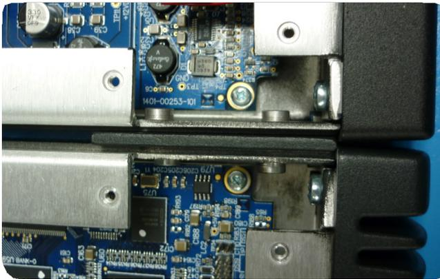
Use the four (4) screws provided with the spacer to secure the two nodes together.
