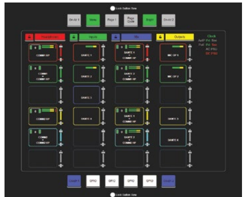
The unit can be fully remotely controlled from the web interface with front-panel lock-out options for every button and encoder.
