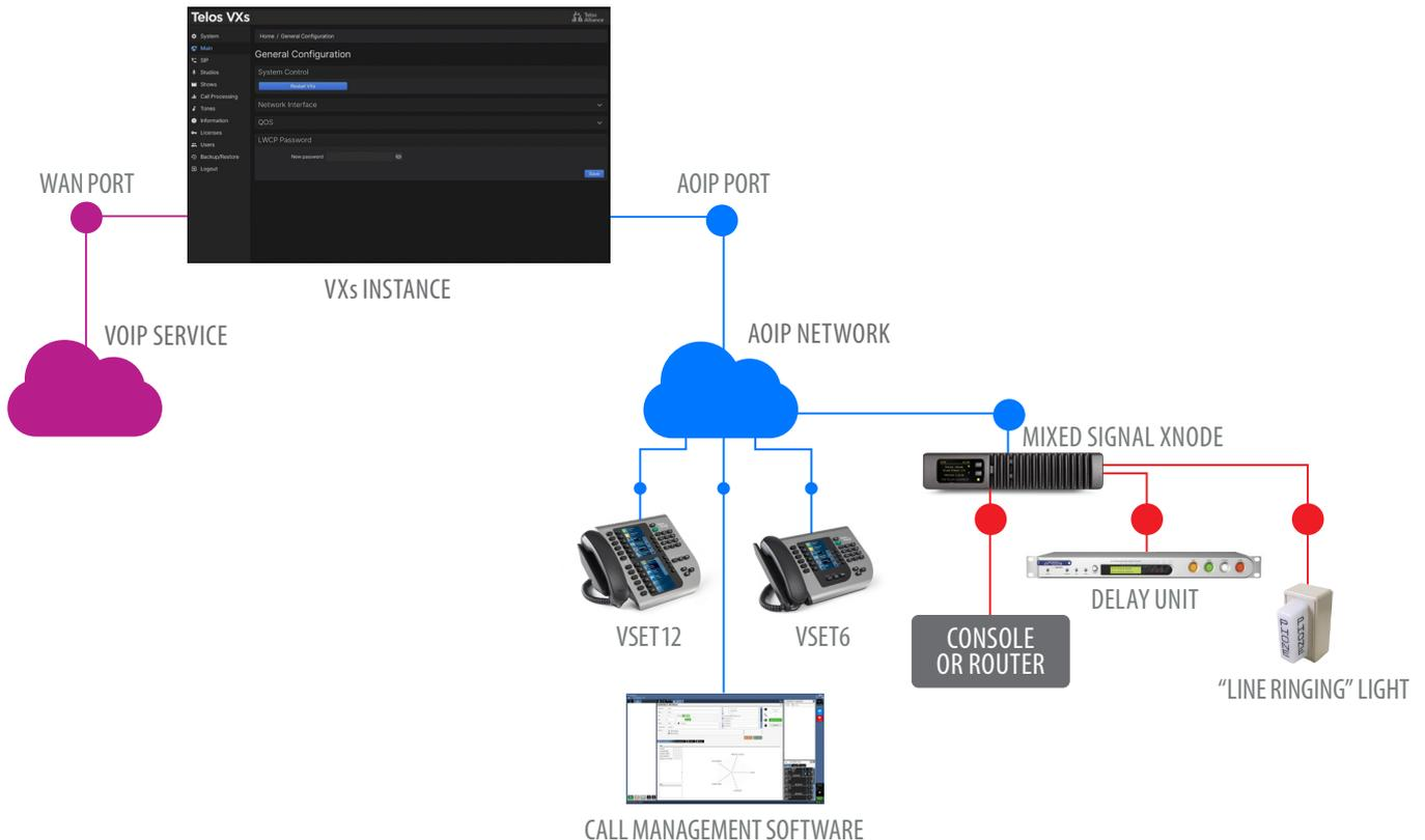
Don't have IP-Audio networking yet? VXs will work with all console brands, networked or not, using Telos Alliance xNodes and the VXs Call Controller drop-in controller for your console. xNodes, like the Telos Alliance Mixed Signal Node, break out audio into analog and digital formats, along with GPIO logic commands. The diagram above shows a typical studio with an analog mixer, using a Telos Alliance Mixed Signal xNode to connect to the console and other broadcast equipment.
