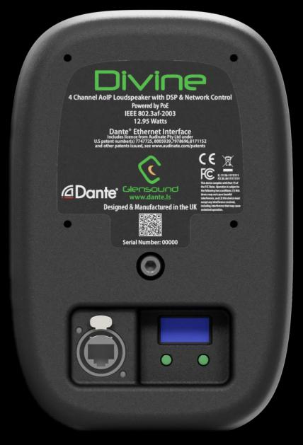
This device uses Audinate's Ultimo Chipset, which can receive 4 incoming audio channels, each at 48kHz. However, this chipset can only receive these 4 audio channels from a maximum of 2 network locations (2 different devices). This is common with any manufacturer that uses this chipset.
