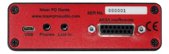
Right view of the PD Dante showing the micro USB AB connector which can be used to power the unit. The unit can be powered by either USB or PoE. Both power inputs can be used together for PSU redundancy. The USB port is also used for firmware upgrades for the PD Dante
