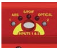
Fig 2-3: RB-DMX4 INPUT 1 & 2 Select Button
