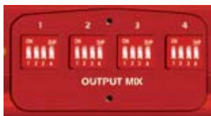
Fig 2-2: RB-DMX4 Front Panel DIPSwitches
