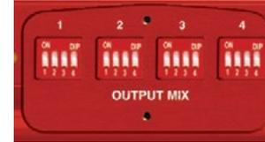
Fig 4-4: RB-DMX4 Front Panel DIPSwitches
