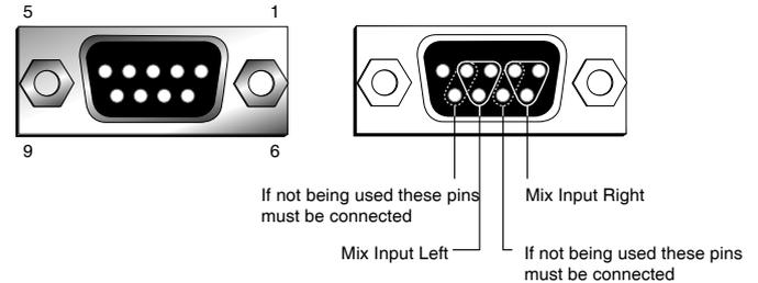
Fig 6-14: RB-OA3 Mix Input Connector Details
