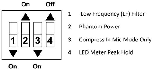
Fig 5-4: DIP Switch to Control Mic & Meter Features
