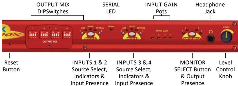
Fig 4-3: RB-DMX4 Front Panel Controls and Indicators
