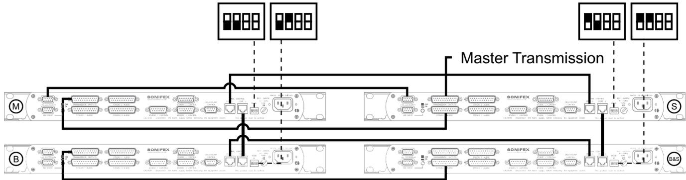
Fig 6-8: RB-OA3 Studio &amp; Bus Expansion Diagram
