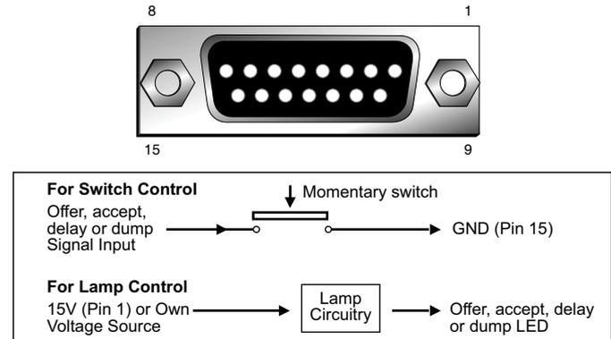
Fig 6-20: RB-OA3 Switch & Lamp Control Details
