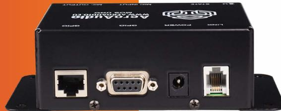
Suitable for signaling of on-air lamps for microphones. e.g. YELLOWTEC MIKA ON-AIR MIC ARM.
