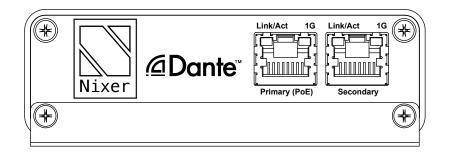
The PLR64 Dante can powered be via PoE (13W) or alternatively be powered via USB (1.5A) by a computer USB port (needs to be a high current port), USB mains adaptor or USB battery pack.
