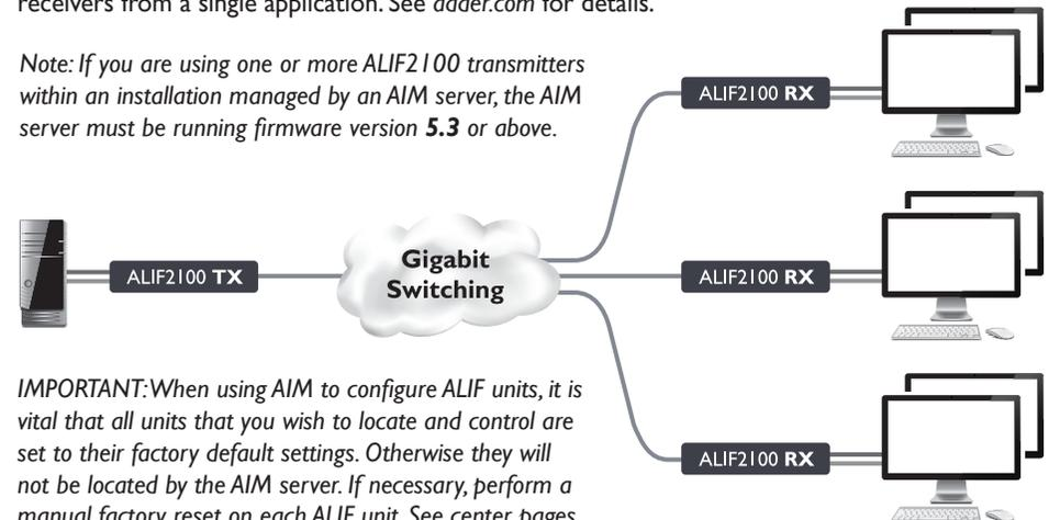
**IMPORTANT:** When using AIM to configure ALIF units, it is vital that all units that you wish to locate and control are set to their factory default settings. Otherwise they will not be located by the AIM server. If necessary, perform a manual factory reset on each ALIF unit. See center pages.
