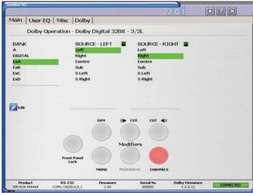
Fig 6-5: Sci Main Screen Showing Dolby Digital Monitoring
