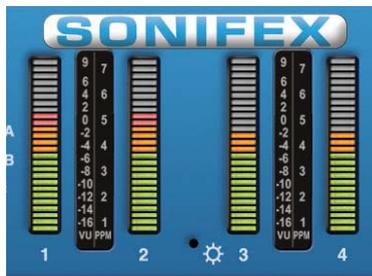
The main meters are quad 26-segment, multicoloured LED bargraphs, displaying the four Sources in the currently selected Bank.
