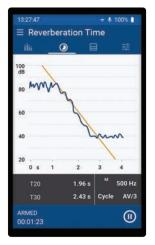
The standard reverberation time measurement determines T20 or T30 in octave bands from 63 Hz - 8 kHz. The values of a measured position or of an entire room are averaged on the XL3. The optional Room Acoustics Package extends the Acoustic Analyzer to 1/3 octave band resolution, T15 or EDT. Use either an impulse source or an interrupted pink noise as the test signal.
