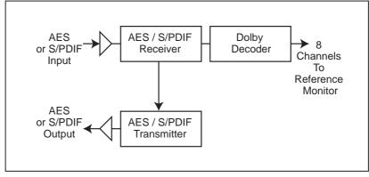
Fig 3-7: RM-E1X/B Block Diagram
