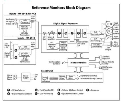
Fig 1-3: Reference Monitor Block Diagram
